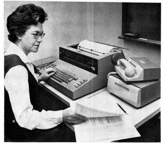
REMOTE COMPUTING CONSOLE in Bldg. 836 is linked to a computer in Los Angeles by long distance telephone lines. Elizabeth L. Frost (2153) demonstrates how the time-sharing system makes it possible to write, edit, compile, execute, and debug a program on the
